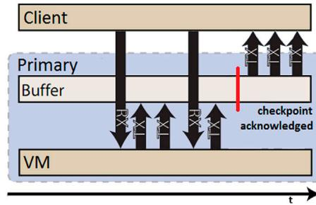
**Figure 2.** Outgoing network traffic from the VM is released after checkpoint synchronisation between primary and backup hosts. Meanwhile, packets are stored into a temporary buffer at the primary host.
