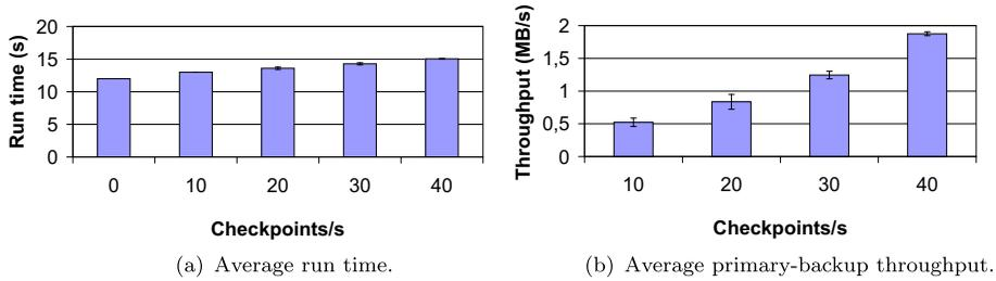
Figure 5. Run time and throughput for CPU benchmark.
