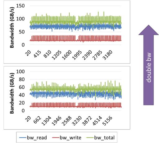
Fig. 8: Results for MILC using full and half risers.
