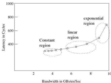
Fig. 1: Memory latency x bandwidth curve. Latency exponentially increases as the amount of bandwidth used by the application approximates the maximum sustained bandwidth. Extracted from [3] and [10].
