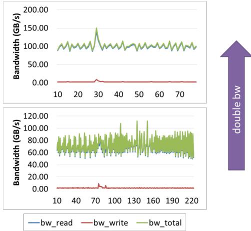
Fig. 7: Results for HPCG using full and half risers.
