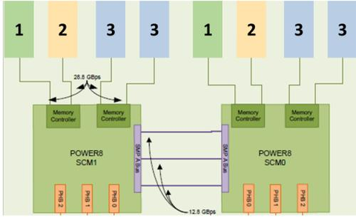
Fig. 4: Detail of Firestone node showing memory risers connected to two POWER8 sockets. Extracted from [17].
