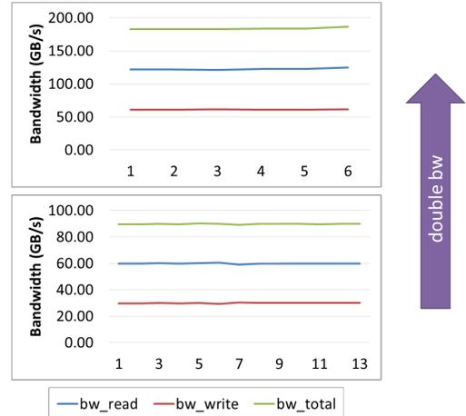
Fig. 5: Results for STREAM using full and half risers.
